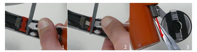
Sharpen the brake flat on the lower side (photo 1) and bevelled on the upper side (photo 2), with a medium grain file, taking care to remove metal filings as they appear on the blade of the brake. To do this, start by sharpening the flat underside, and then gently work your way to the upper side of the blade. To check how sharp the blade is, pull the metal strip back firmly with a pair of pliers: the brake should stop the metal strip from moving back (photo 3).
