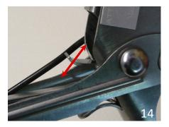
Check that the metal strip is feeding correctly and that the cut is occurring at the correct moment of the closing cycle.
