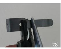
The tension of the spring blade is adjustable; this requires taking it apart and reshaping it using pliers (photo 28).
