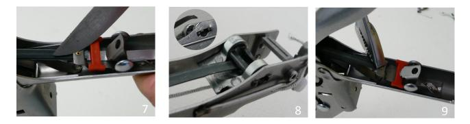
**1**- Remove the rivet using a knife (photo 7) and remove the worn blade.
